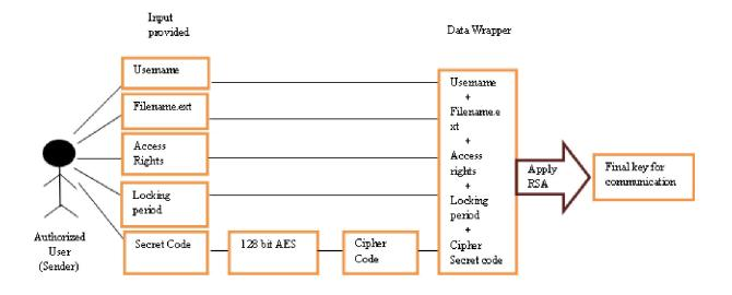
Fig. 1. Encryption Process at sender side.
