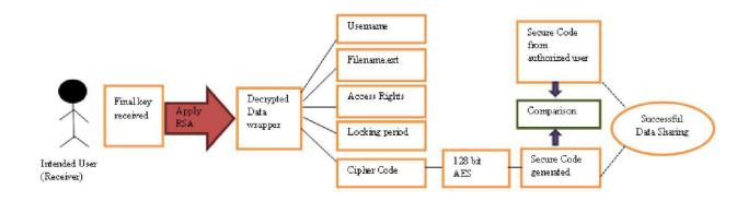
Fig. 2. Decryption Process at receiver side
